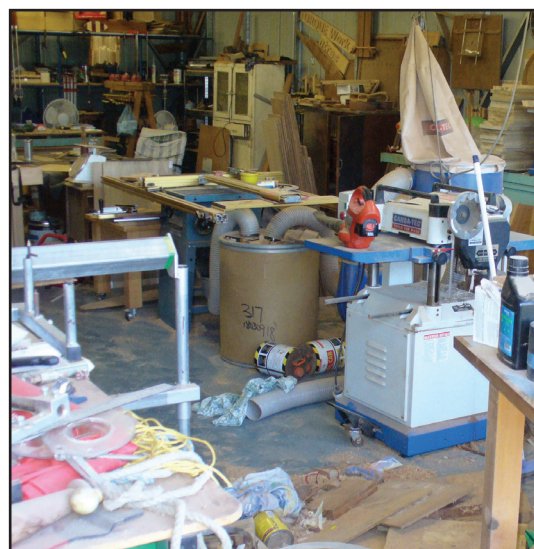
Poor housekeeping is the main source of slips, trips and falls in the workplace
